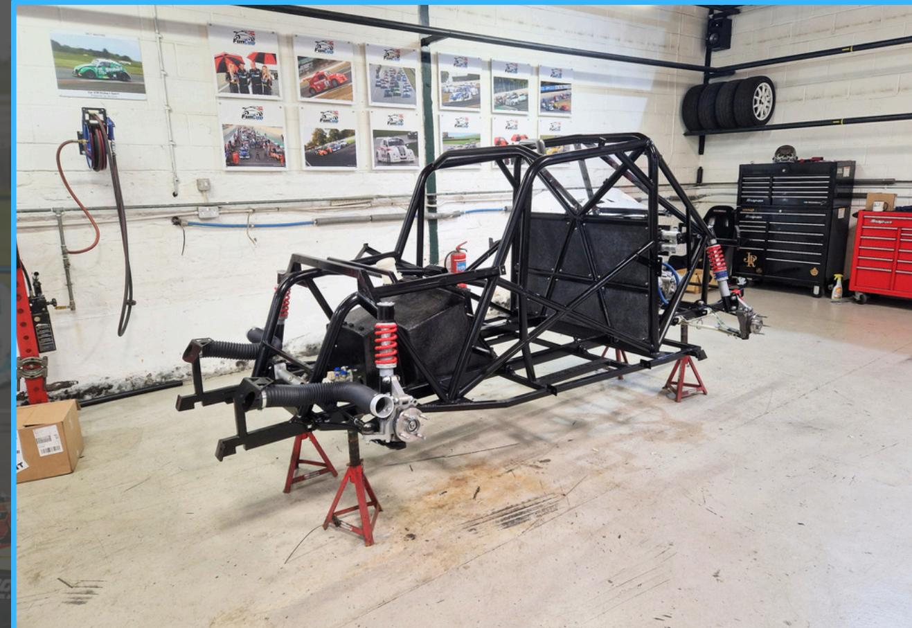
The cars are race designed, with a super strong space frame chassis. They are powered by an 1800cc, 133 bhp VW/Audi petrol engine, with the ultra reliable Sadev sequential gearbox with paddle shift. Pit-to-car radio are also available as optional extras and they all feature race brakes and fully adjustable suspension.
