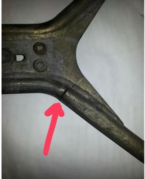
It is recommended lifing the rear wishbones to avoid failure.
