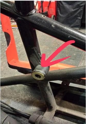
Please inspect the condition of the gear lever mounting bracket, we have seen this bracket fail and break off the chassis since the introduction of the sequential gearbox. Weld and brace if required and inspect on a regular basis.
