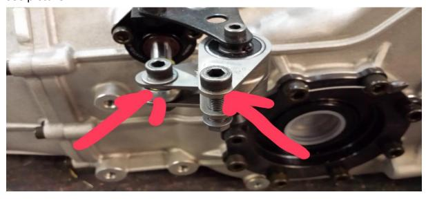
2. It is also recommended that you remove and inspect the right engine mounting, check for any signs of cracking, either replace or repair/strengthen as required. Please see picture:
