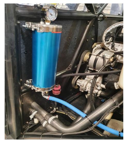
The oil accumulator will maintain oil pressure in all high speed/high grip corners. We recommend this option to avoid any loss of oil pressure. The recommended pressure is 3.5 Bar. Part No. O/acc1 this is listed on the website under options.
